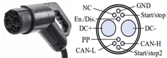
Fig. 5.27 CHAdeMO plug [11] and pin descriptions
