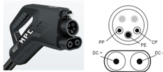
Fig. 5.29 CCS 1 DC charging plug and pin descriptions [10]
