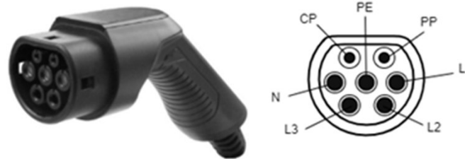
Fig. 5.24 Type 2 AC plug [7]
