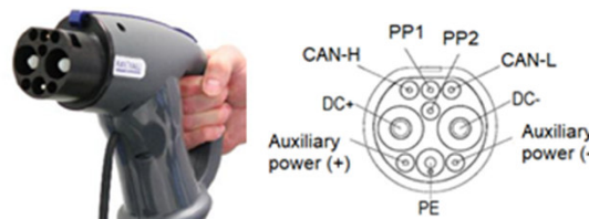
Fig. 5.28 GB/T Plug and pin descriptions [12]
