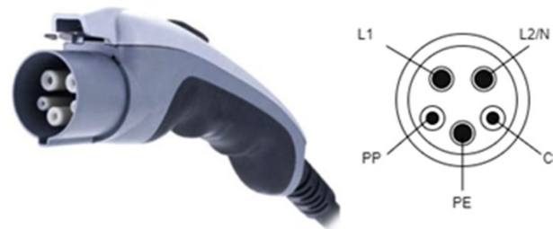
Fig. 5.23 Type 1 AC plug [6]
