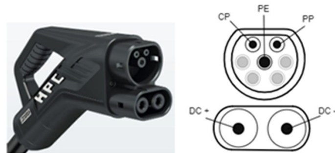
Fig. 5.30 CCS 2 Charging plug and pin descriptions [10]
