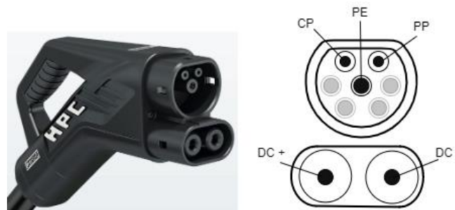
Fig. 5.30 CCS 2 Charging plug and pin descriptions [10]
