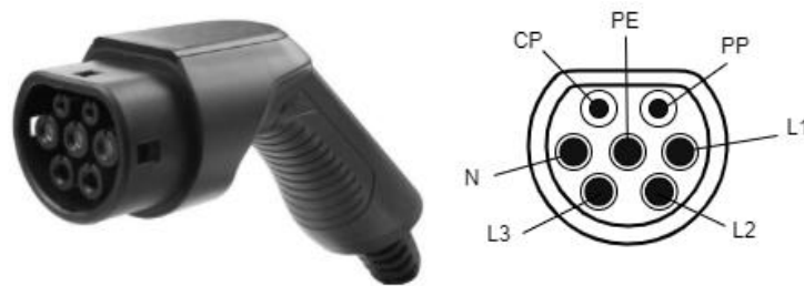
Fig. 5.24 Type 2 AC plug [7]
